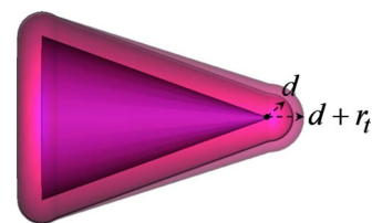
FIG. 23. (Color online) Cloaking cover for the silver cone locally thicker around the tip.
